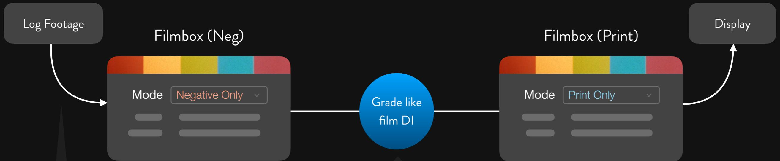
Grading between the two Filmbox nodes now behaves like grading a scan of camera negative film in a film DI.
